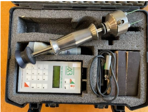
Fig. 4. Brookhuis wood moisture content measuring device used for indicative measurements
