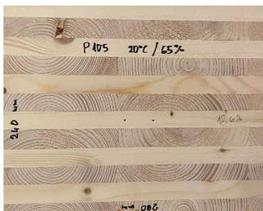
Fig. 1. Group 1 sample lay-up, exposed end-grain 50.0% ( n = 8 )
