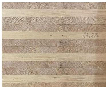
Fig. 2. Group 2 sample lay-up, exposed end-grain 64.8% ( n = 5 )
