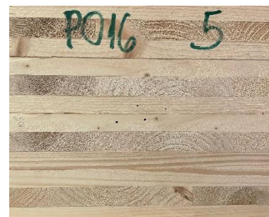
Fig. 3. Group 3 sample lay-up, exposed end-grain 34.5% ( n = 5 )
